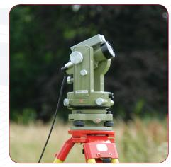
(Measurement resolution is limited by the prevailing geomagnetic conditions, the skill of the operator and the mechanical stability of the tripod, if used.)
