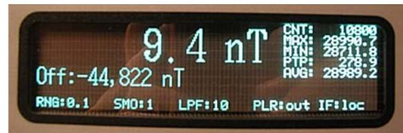
A total of 16,384 data points can be stored in the buffer, which represents a little over 90 minutes of data. The data stored in the buffer can be plotted on the VFD display for immediate viewing and analysis.
