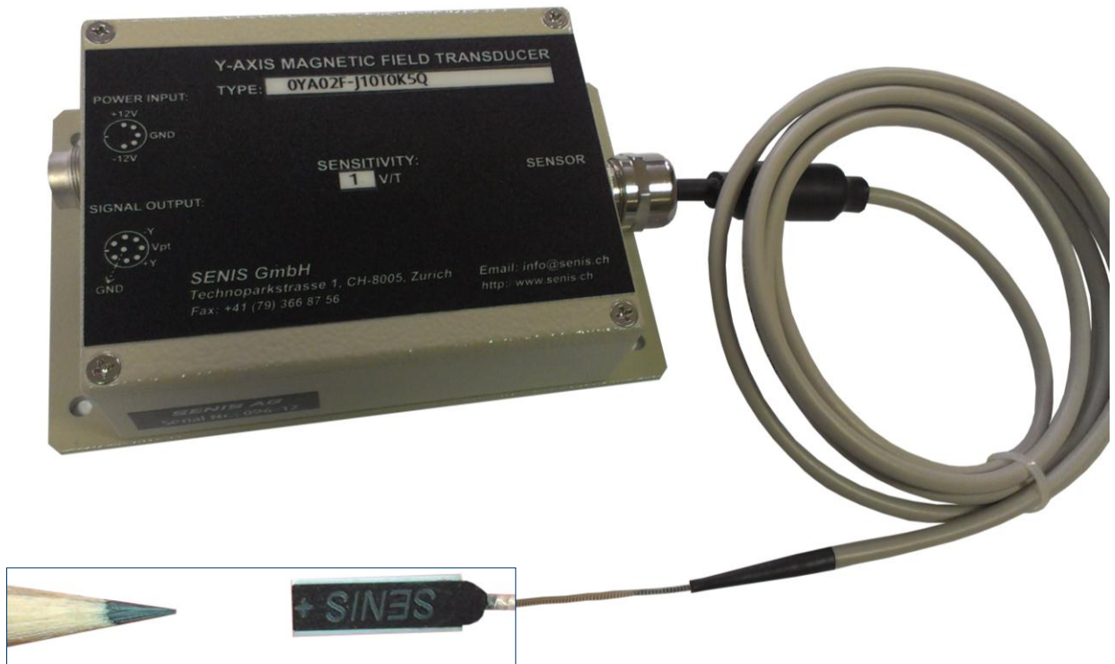
Figure 2. Photo of a 1-axis magnetic field transducer with integrated Hall Probe
